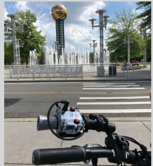
A C3FT (pronounced "see three feet") ultrasonic device mounted on a KPD police bicycle.
