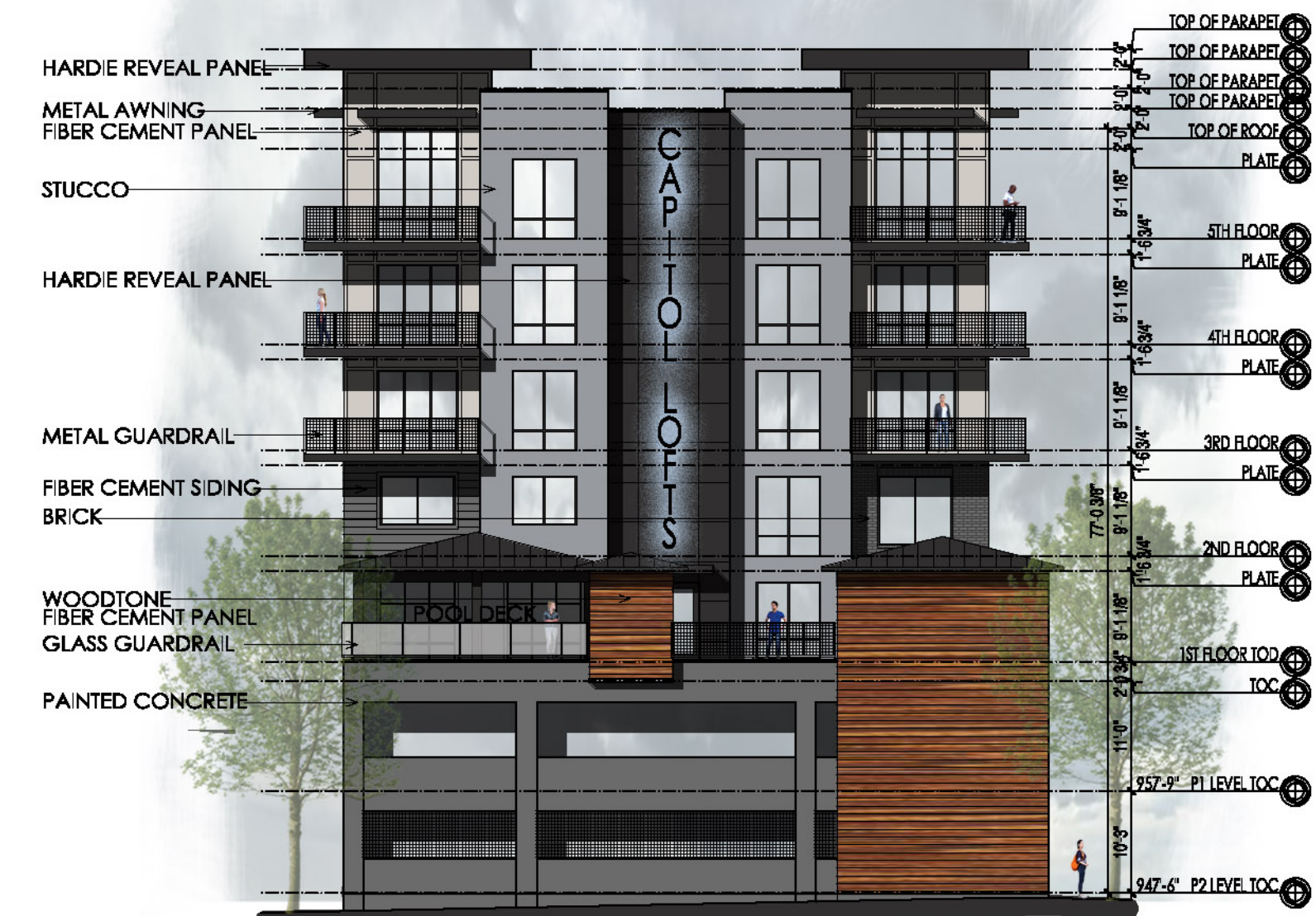
3 BLDG ELEVATION - WEST SCALE 1/16"=1'-0"
