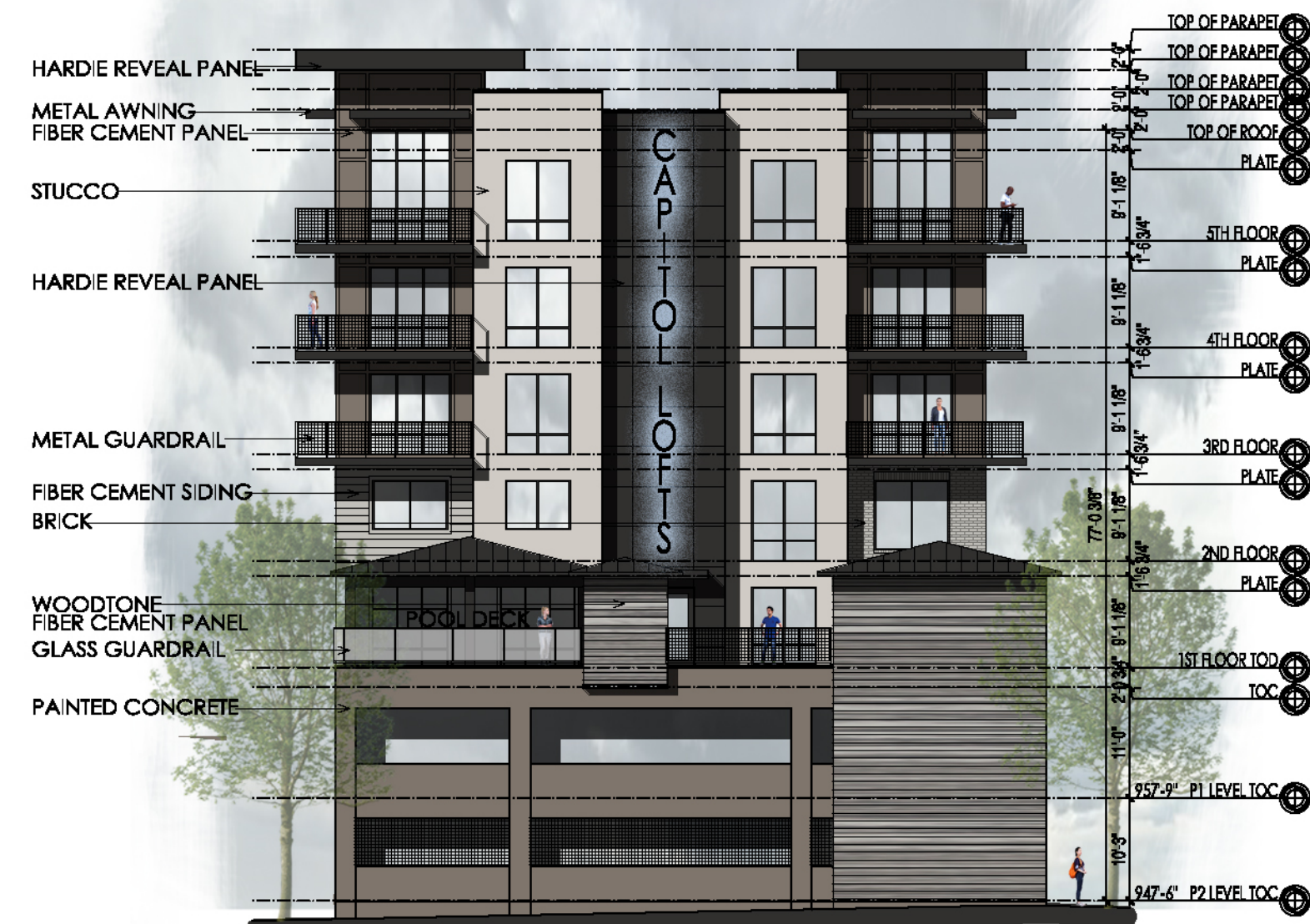
3 BLDG ELEVATION - WEST SCALE 1/16"=1'-0"
