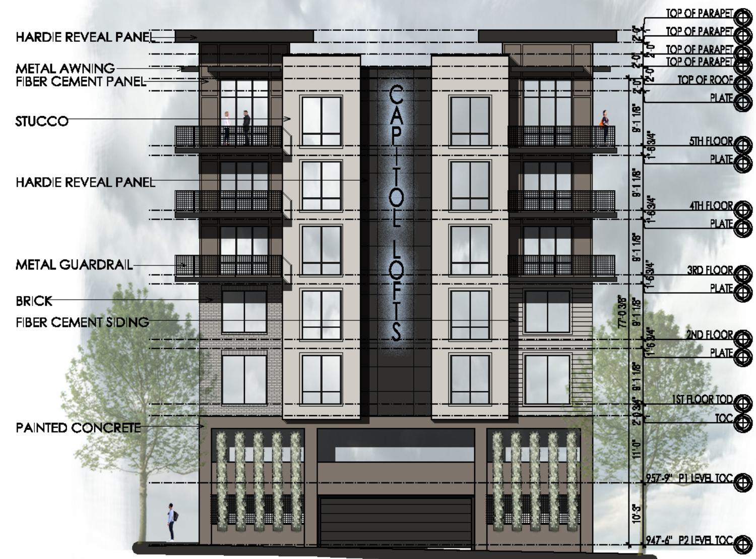
2 BLDG ELEVATION - EAST SCALE 1/16"=1'-0"
